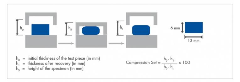
The specimen is compressed by 25%. The compressed specimen is heated to the test temperature. DIN ISO 815 discribes two methods.
